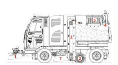
The waste is collected thanks to the mechanical action of the side (1) and central (2) brushes and the vertical conveyor (3). Suction (4) is intended to capture dust as soon as it is raised from the ground. Optimised suction for complete dust suppression thanks to the large surface filter (5).
