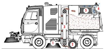
The waste is collected thanks to the mechanical action of the side (1) and central (2) brushes and the vertical conveyor (3). Suction (4) is intended to capture dust as soon as it is raised from the ground. Optimised suction for complete dust suppression thanks to the large surface filter (5).
